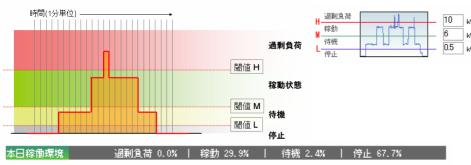
Summarizes the operation status of each equipment in following 4 statuses [overload] , [running], [standby], [off]
